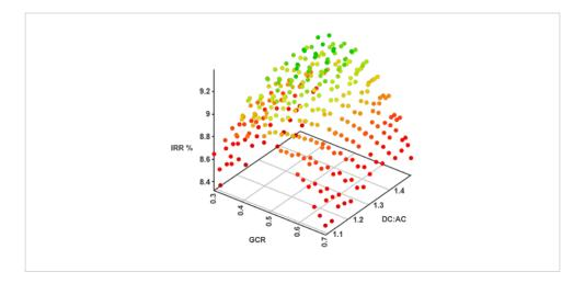
SIFT generated heat map of hundreds of layout configurations, representing the trade-off between the row spacing (GCR), DC:AC ratio and rate of return (IRR%).
