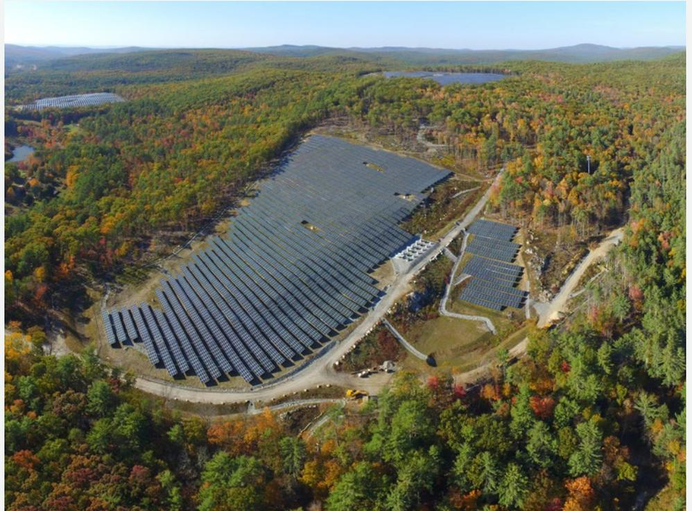
Solar developer Borrego Solar engaged Terrasmart to install the solar foundation for a 7.3 MW project in Orange, Massachusetts. When assessing the site, the installation team noticed some challenges that would make foundation installation difficult—a 21% north and south slope, rocky terrain, and drainage swales.
