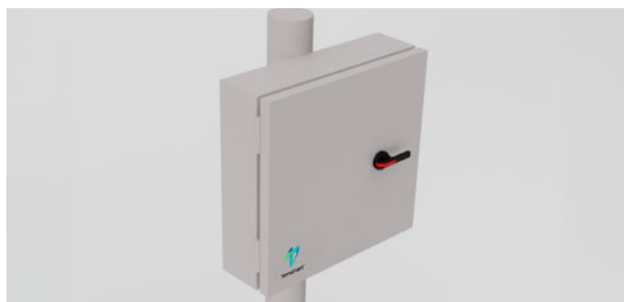
Floating Disconnect Combiner, 1500VDC, 275A disconnect, 15 input circuits, transient surge protection, NEMA-4X fiberglass enclosure
